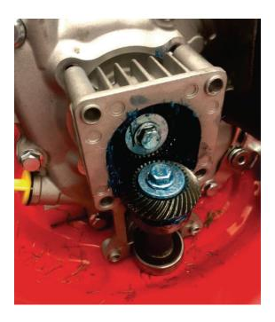
Figure 6 does not demonstrate that the power is transmitted from the vertical drive shaft directly to the mower blades. It shows how the shafts are placed, but it is not sufficient evidence to demonstrate that power can only be transmitted from the vertical drive shaft to the blades of the lawn mower.
