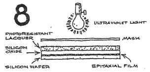
Over the epitaxial film, induce a silicon oxide coating. Over that, place another coating of a "photoresist" lacquer. Over that, place a "mask" with the desired electronic pattern. Now expose the surface to ultraviolet light.
